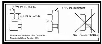
Handrails are required on at least one side when stairways have four or more risers.
